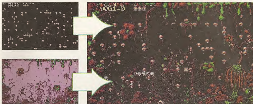
This Amigaified Centipede reserves one playfield for the backdrop, confining game action and collision detection to the other playfield
